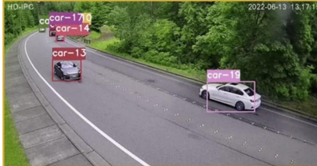
Vehicle detection, tracking, counting
