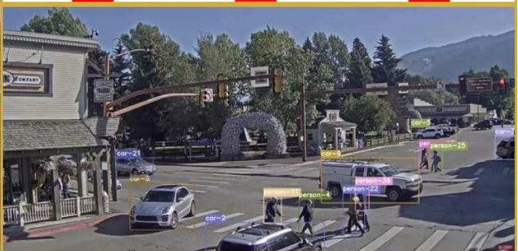
Multi-modal detection (car, truck, bus, pedestrian, cyclist, scooter, etc.)
